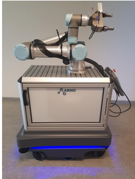
Figure 2: Heron in manual (joystick) driving mode with status blue color.
